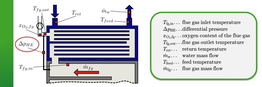
→ utilization of **fast differential pressure measurement**
