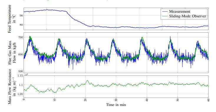
→ high accuracy even during steep change of feed temperature 22.01.2020
